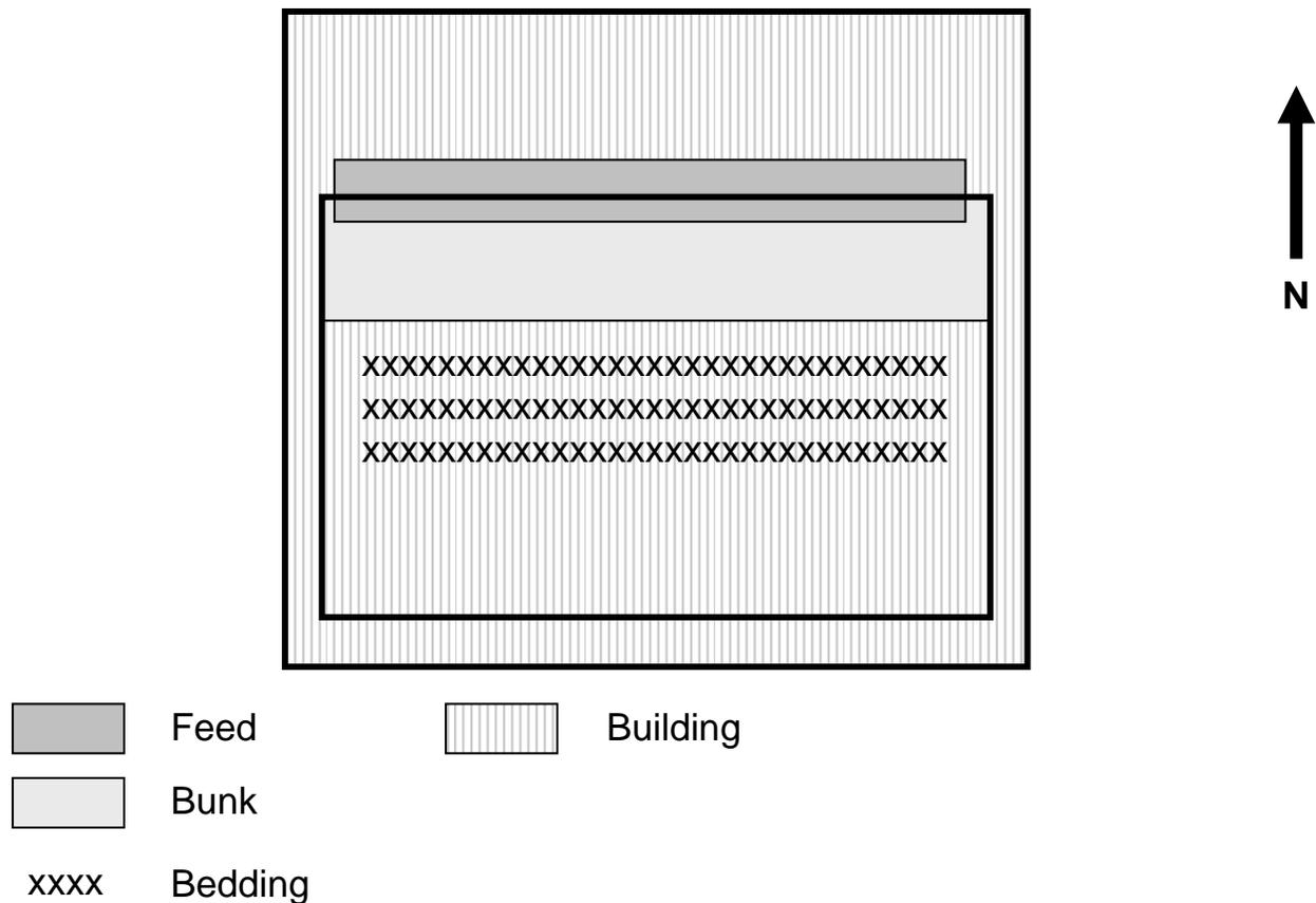
Figure 3. Confinement lot with solid floor. Cattle are under a building that is protected to the N, but may or may not have side walls. In spite of being indoors, it is recommended that cattle be bedded to keep clean and dry.
