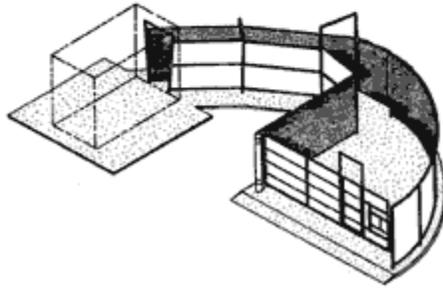
Figure 12. Examples of curved working alleys
