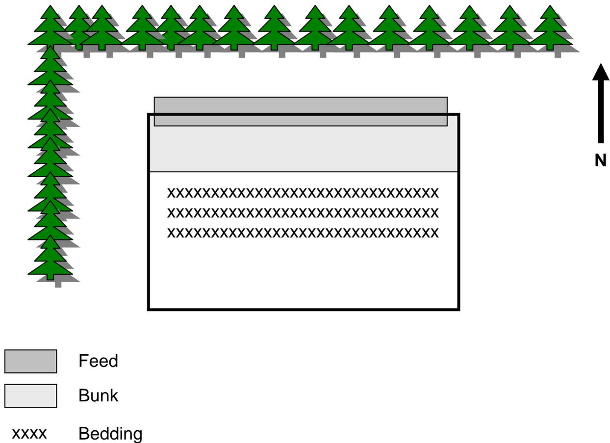
Figure 1. Open lot with shelter belt. Shelter belt should be at least 50' from lot. Windbreaks and mounds may also be built within the lot as needed. Lot should slope away from bunk at 4% to 6%. Drainage diversions should run away from the bunk, from N to S in this drawing.
