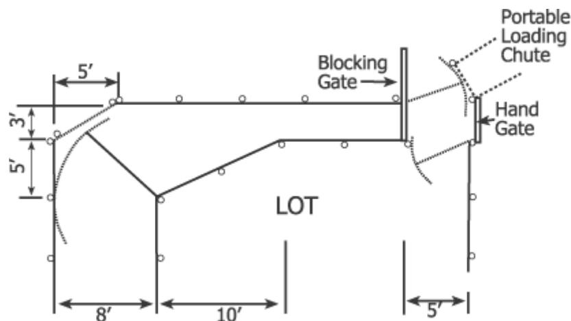
Figure 8. A basic working facility design is depicted with loading chute, and holding pens.
