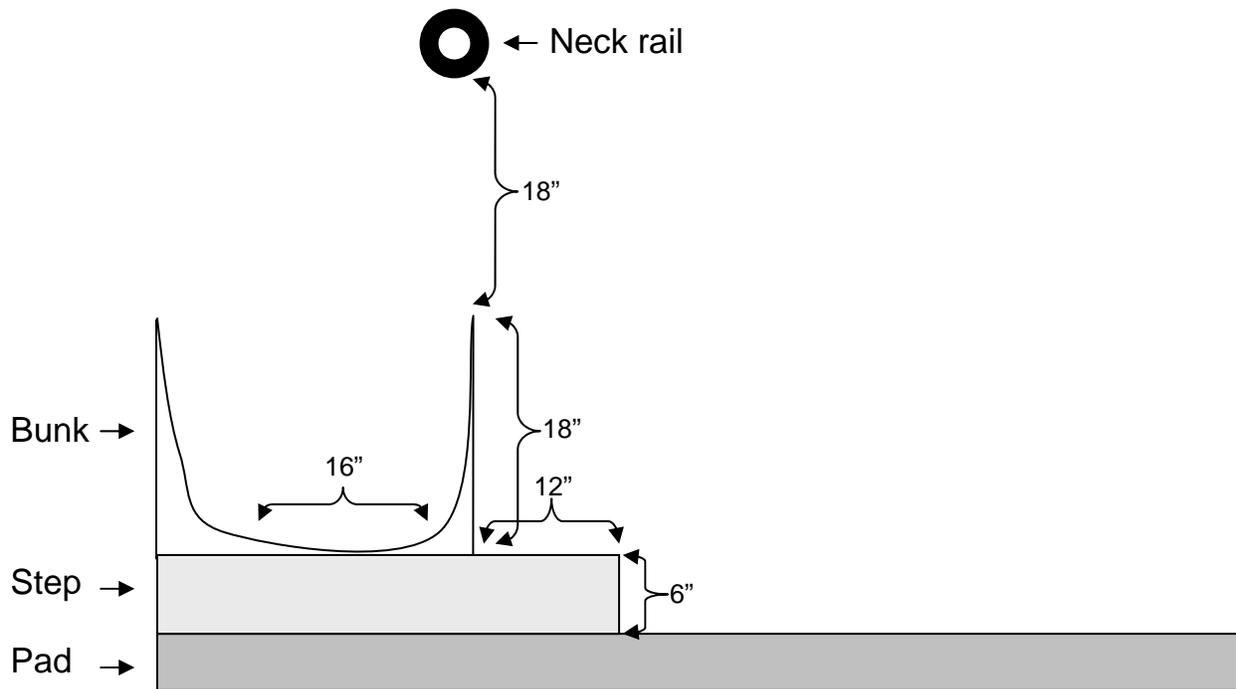
Figure 4: Recommended dimensions for feed bunk.
