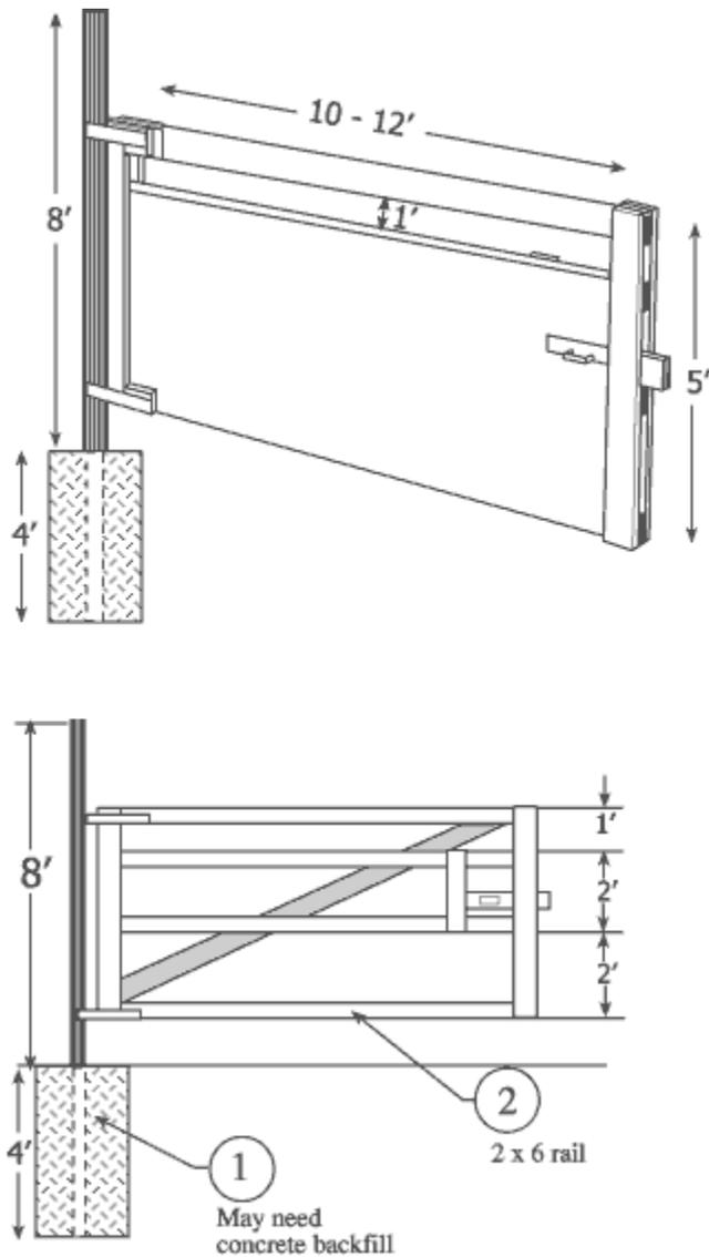
Figure 11. Example of a Solid-Sided Sweep Gate
