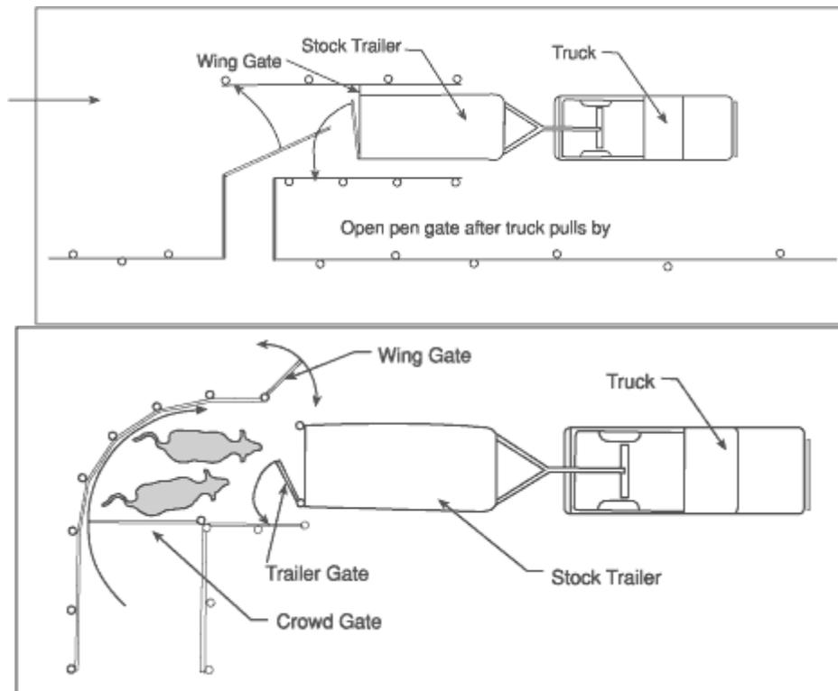
Figure 13. Some examples of loading chutes for livestock trailers
